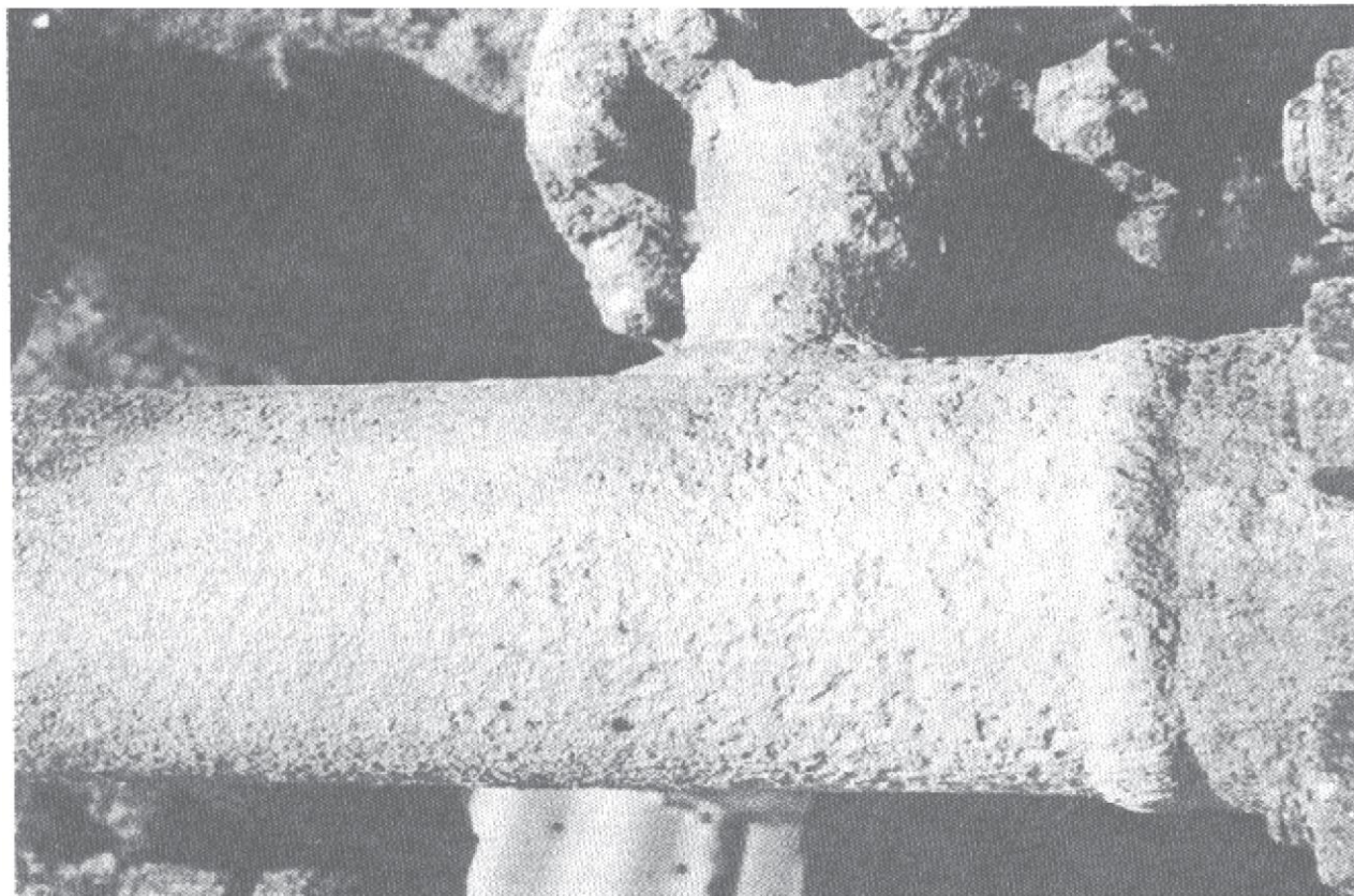
Figure 20—Severe Atmospheric Corrosion of Piping
